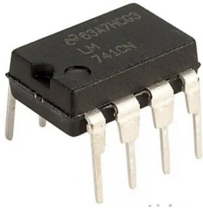
(a) An operational amplifier (LM741).
